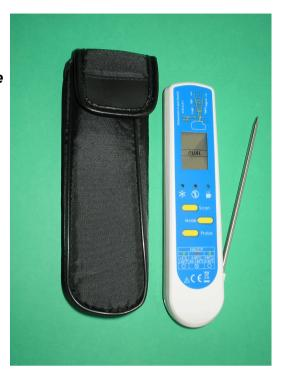
The RT303 DUAL Thermometer is very handy because it offers two functions in one: Infra red measurement as well as a very accurate fold-out probe. The user can choose the function by pressing the relevant button.
